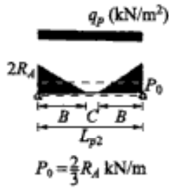
Figure 3.22. Reactions due to load q_p on landing.
